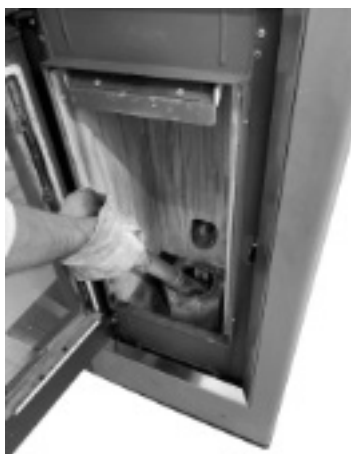
Fig. 34 - Burning pot box cleaning
