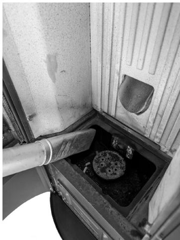
Fig. 38 - Burning pot box cleaning
